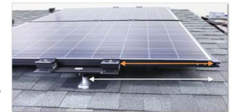
Double Mounting Assembly enables the mount to be up to 26" from the end of the module, while maintaining the 19" cantilever.
